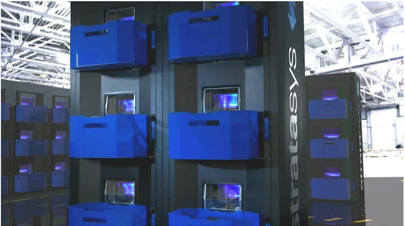
The Stratasys Continuous Build 3D Demonstrator automatically cues jobs to print, ejects completed parts and starts the next job without interruption, increasing efficiencies and opening up more time for tasks unrelated to managing the 3D printing process. [Learn more.](#)
