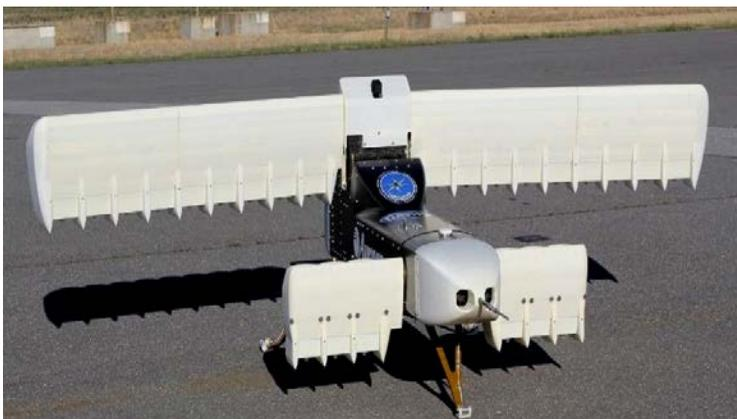
Aurora Flight Sciences 3D printed major portions of its scaled LightningStrike vertical takeoff/landing demonstrator.
