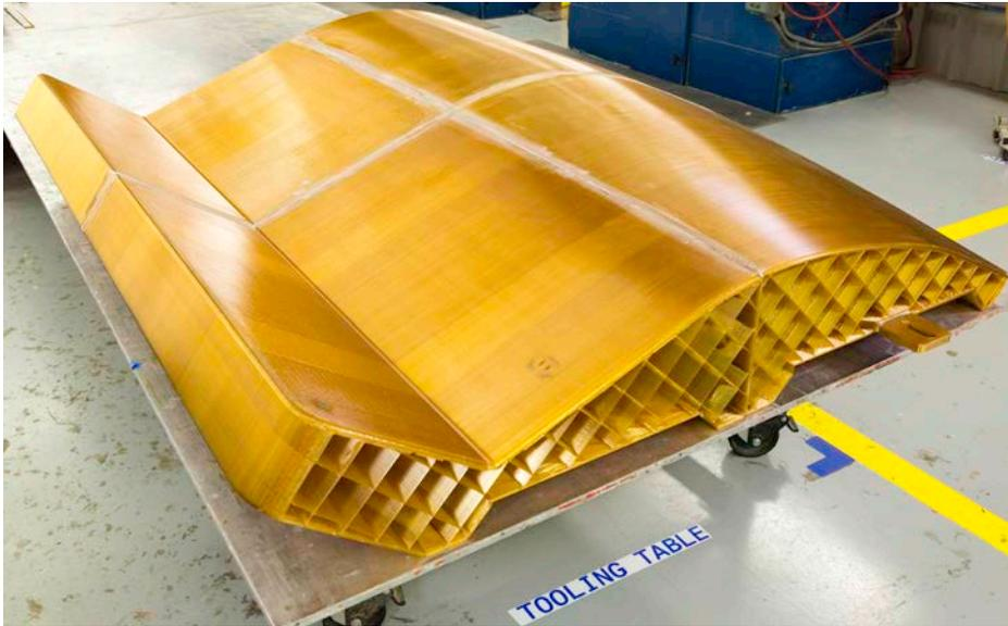
FDM technology simplifies the fabrication of composite layup mold and sacrificial tooling while providing more design freedom. [Learn more.](#)
