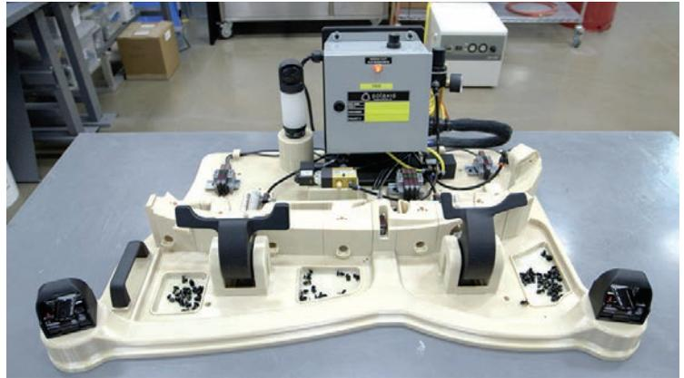
Solaxis created an automotive assembly jig with 3D printing, cutting weight and improving accuracy. [Learn more.](#)
