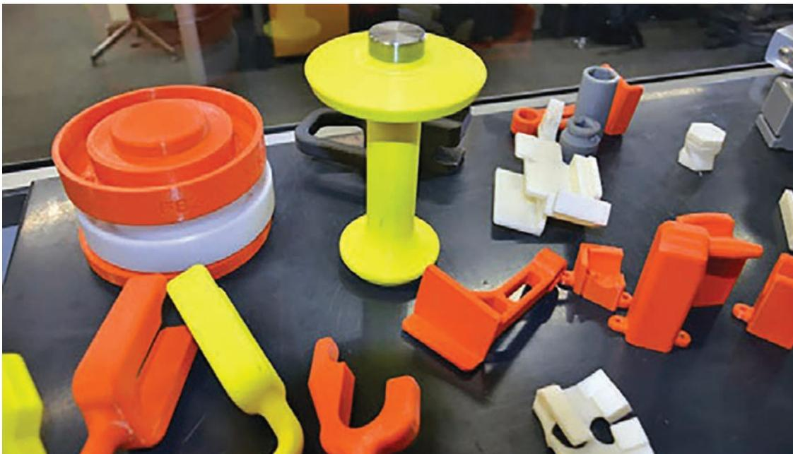
Volvo Trucks replaced metal tooling for its engine production facility with lighter 3D printed tools and fixtures. [Learn more.](#)
